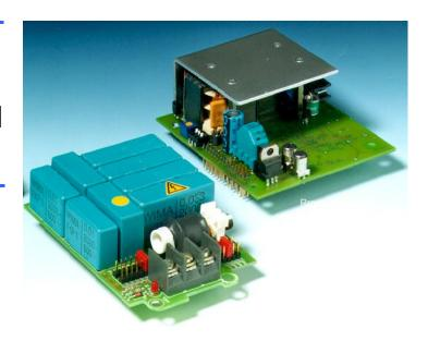
interface between the 134.2 kHz HDX/FSK transponder and the Data Processing Unit. It sends an energizing signal to the transponder, modulates the RF signal to send data to the transponder, receives the identification signal and processes it for digital decoding.
